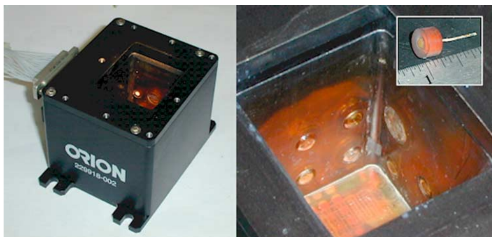
Figure 1. The Mars Environmental Compatibility Assessment wet chemistry lab ion-selective electrode (ISE) sensor array showing the internal placement of individual sensors. Inset shows a typical individual ISE sensor.
