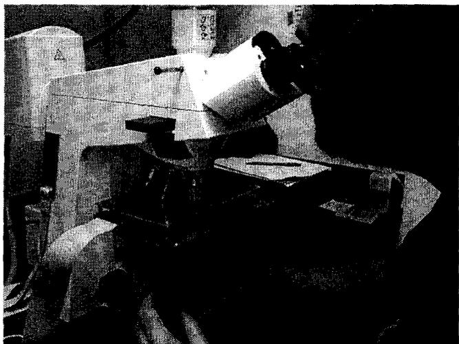
Figure 3. E-Tongue 3 with its top cover attached is placed on the stage of a Zeiss Axioplan microscope.
