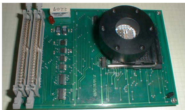
Figure 8. E-Tongue 2 electronics apparatus fabricated on a 10-cm by 15 cm printed circuit board.
