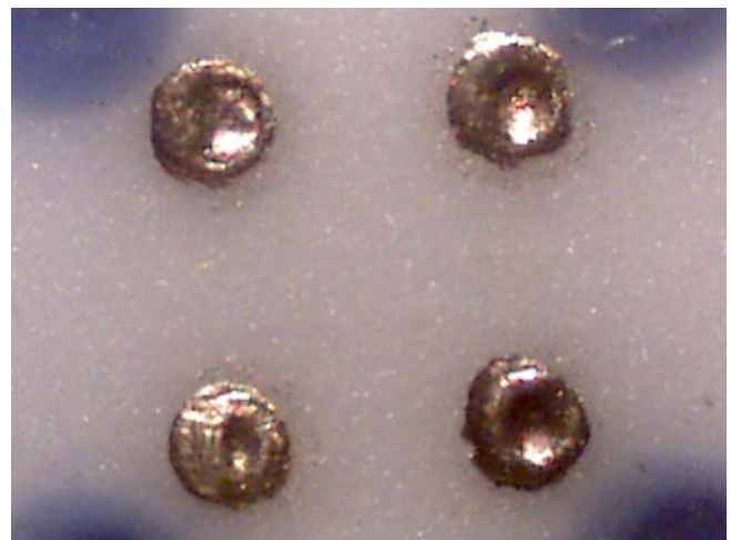
Figure 5. Photomicrograph of the conductivity sensor where the electrode spacing is 1.25 mm.
