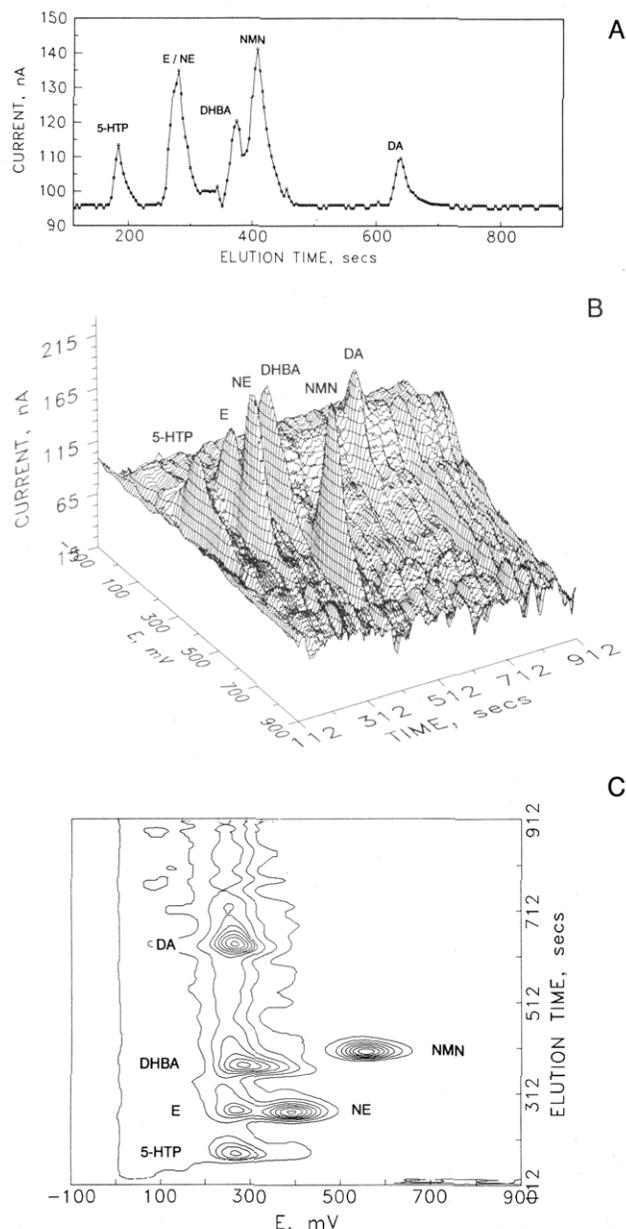
**Figure 3.** (A) Standard chromatogram of sample containing 5-HTP, E, NE, DHBA, NM, and DA, all at  $1 \times 10^{-6}$  M, with the CFE detector potentiostated at 650 mV. (B) Same sample analyzed with the chromatovoltammetric technique as a three-dimensional plot and (C) as a isogalvanic contour plot.
