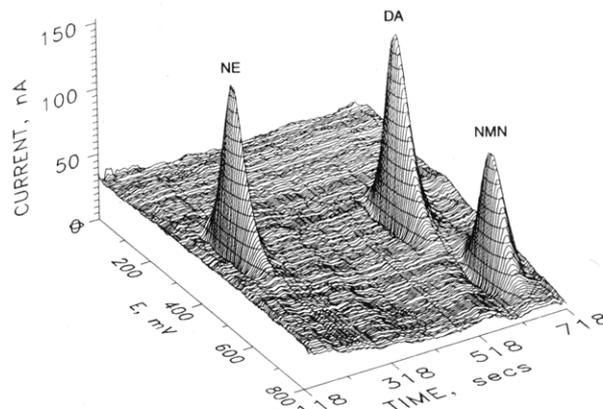
**Figure 2.** Square wave chromatovoltammogram of NE, DA, and NM, all at  $1 \times 10^{-5}$  M, represented as a three-dimensional XYZ plot. Chromatographic and voltammetric conditions are given in text.
