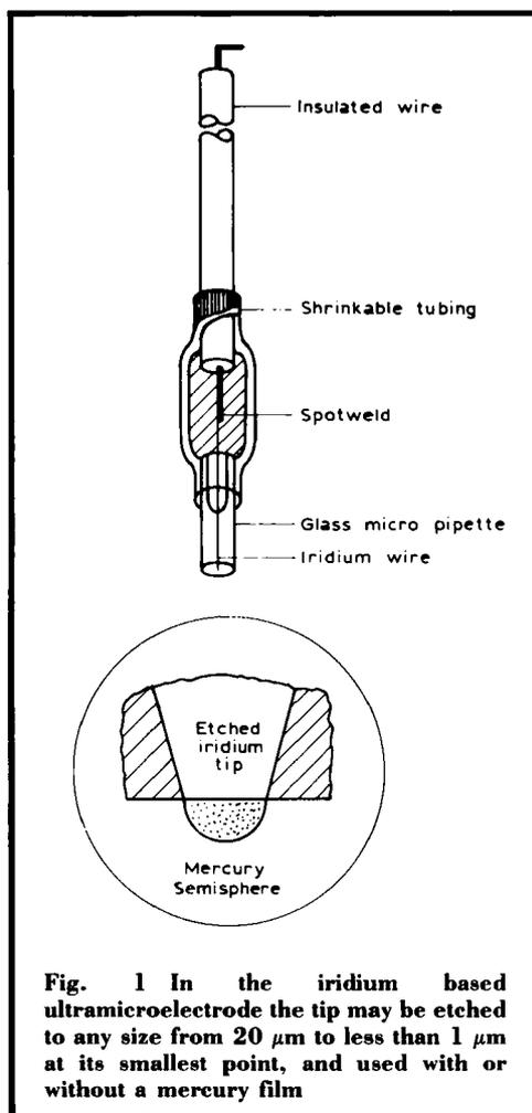
Fig. 1 In the iridium based ultramicroelectrode the tip may be etched to any size from 20  $\mu\text{m}$  to less than 1  $\mu\text{m}$  at its smallest point, and used with or without a mercury film
