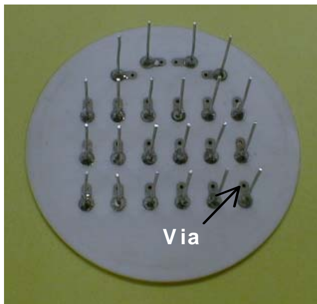
Figure 2b. Ceramic substrate, bottom view, showing the pins used to connect to the top side electrodes through the vias.
