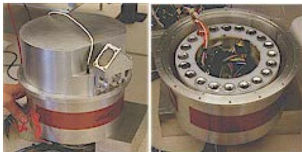
The RCAL expands on the MECA concept by providing twenty individual sealed sample chambers mounted on a rotating carousel. The soil, after delivery by an external mechanism such as a robotic arm or sub-surface drill, is loaded into a dual soil hopper. Multiple small samples can then be taken from the hopper and delivered to the test chambers. After the chamber is punctured, one of a set of four electrodes mounted over the carousel can be inserted into the selected chamber.
