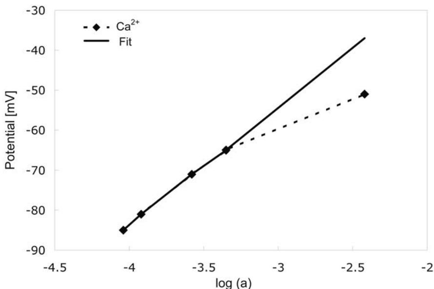
**Figure 8.** Calibration of  $\text{Ca}^{2+}$  in the presence of  $8 \times 10^{-5}$  M perchlorate by standard addition of 1 M  $\text{CaCl}_2$ . The response is Nernstian (29 mV/decade) only between  $10^{-5}$  and  $10^{-3}$  M.
