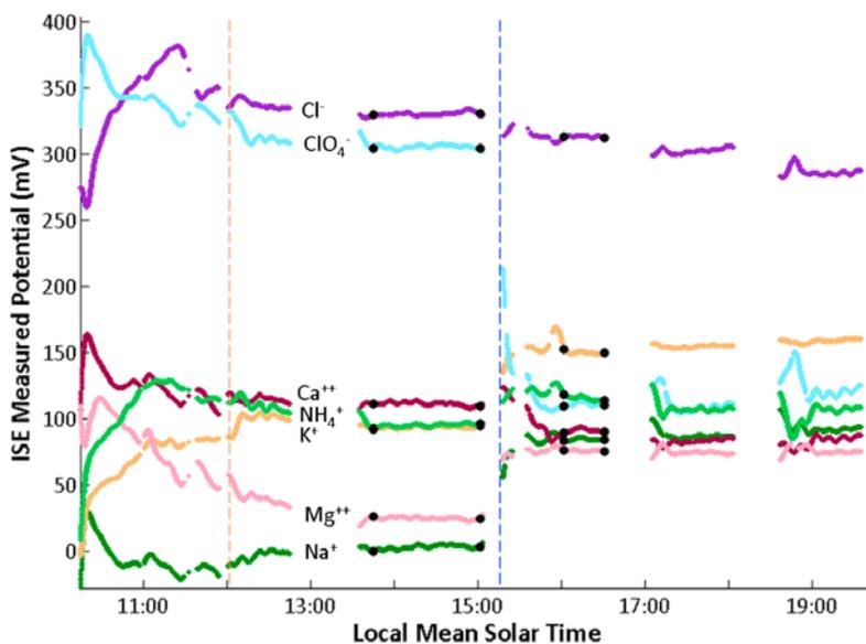
**Figure 5.** Sensors response for the analysis of the Sorceress 2 sample on sol 107 in cell 2. The two vertical lines indicate the addition of the calibrant crucible and the soil sample. The x axis indicates the sol and local mean solar time. Cations and anions show a positive and negative potential change, respectively, for an increase in concentration.
