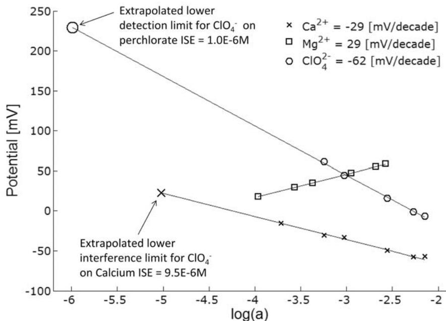
**Figure 7.** Calibration of the Hofmeister ISE (formally  $\text{NO}_3^-$  ISE) using standard additions of 0.5 M  $\text{Mg}(\text{ClO}_4)_2$  into a calibrant equivalent solution (TS21). An extrapolation of the results yields the activity lower detection limit of  $1.0 \times 10^{-6}$  M for the WCL perchlorate sensors. The value is substituted in equation (2) to determine the calibration intercept.
