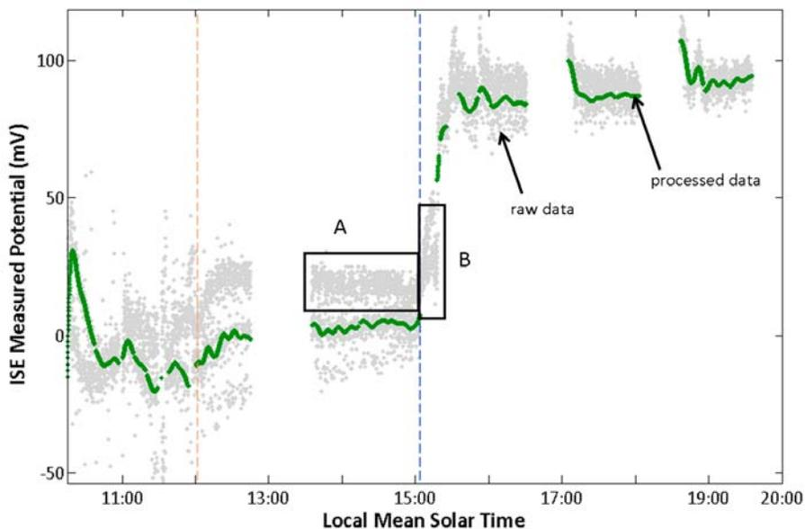
**Figure 2.** Processing of a particularly poor signal for Sorceress 2 on sol 107. Points in region A exemplify points adversely affected by the ORP fluctuations that resulted from temperature measurements. They were easily identified by the bimodal distribution and were removed. The points in box B were removed since they were adversely affected by large thermal and ORP fluctuations due to drawer open and close events. The remaining data were filtered, resulting in the final processed signal.
