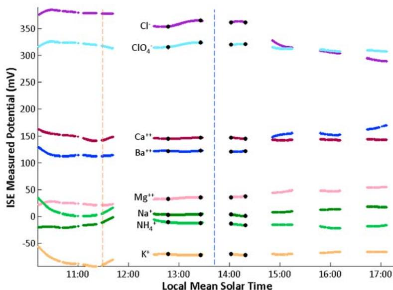
**Figure 6.** Sensors response for the attempted analysis of the Golden Goose sample on sol 96 in cell 3. The two vertical lines indicate the addition of the calibrant crucible and the soil sample. The x axis indicates the sol and local mean solar time. Cations and anions show a positive and negative potential change, respectively, for an increase in concentration.
