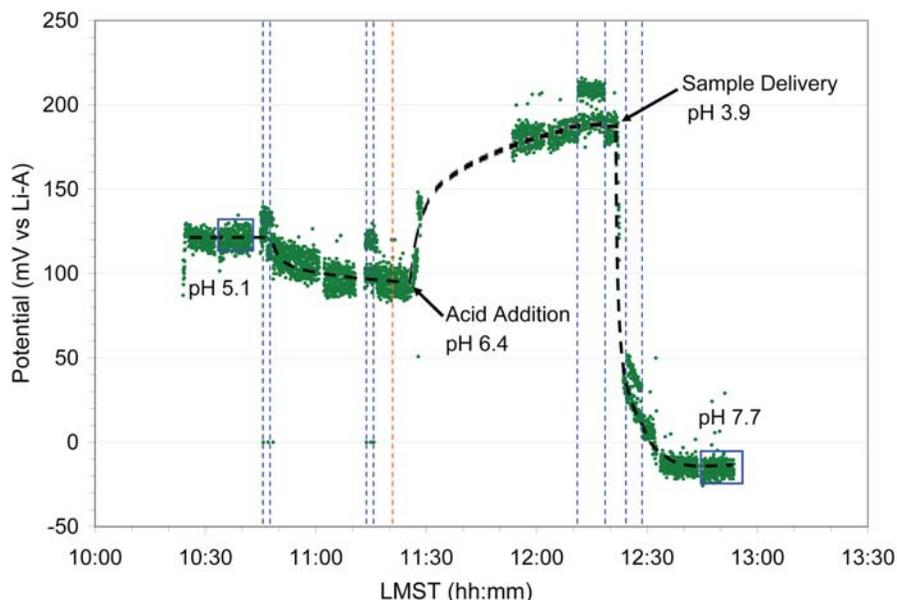
**Figure 9.** Response of the pH1 sensor for the Sorceress 1 soil sample on sol 41. The four pairs of dashed blue lines indicate the opening and closing of the drawer. The orange dashed line indicates the delivery of the crucible containing the calibrant. The blue boxes enclose the interval used to determine the initial calibration pH and the sample pH. LMST is the local mean solar time.
