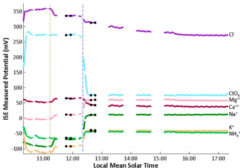
**Figure 3.** Sensors response for the analysis of the Rosy Red sample on sol 30 in cell 0. The two vertical lines indicate the addition of the calibrant crucible and the soil sample. The x axis indicates the sol and local mean solar time. Cations and anions show a positive and negative potential change, respectively, for an increase in concentration.
