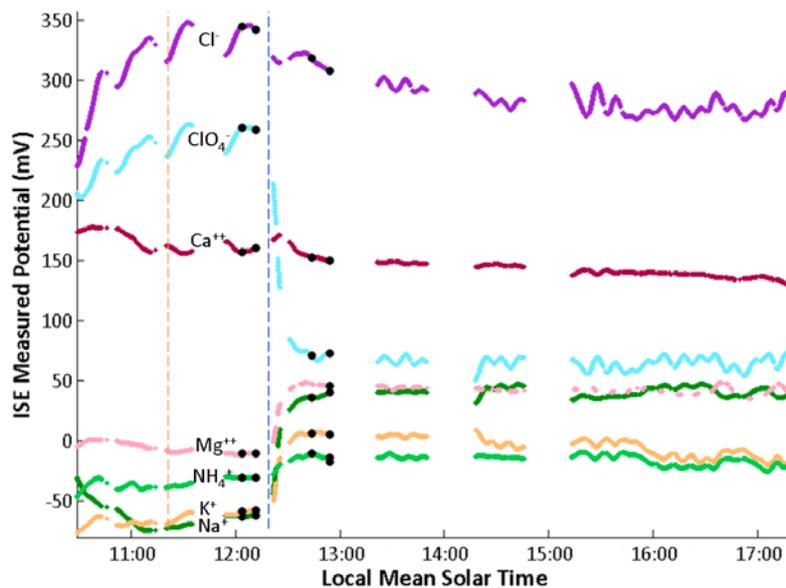
**Figure 4.** Sensors response for the analysis of the Sorceress 1 sample on sol 41 in cell 1. The two vertical lines indicate the addition of the calibrant crucible and the soil sample. The x axis indicates the sol and local mean solar time. Cations and anions show a positive and negative potential change, respectively, for an increase in concentration.
