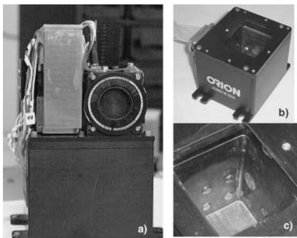
Figure 1. A view of the MECA WCL components showing a) the actuator assembly containing the water reservoir, sample drawer, and WCL, b) the lower cell, and c) a close up of several sensors mounted on the interior of the WCL.
